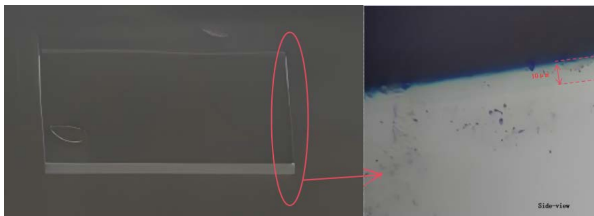
Figure 2. Lithium niobate slab waveguide physical prototype
